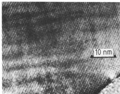
**Figure 4** An image of a crystal flake from crushed  $\text{BaAl}_2\text{Ti}_6\text{O}_{16}$  after prolonged electron irradiation. Minor irregularities in the images correspond to small changes on the local scale of the angle  $\beta$ .
